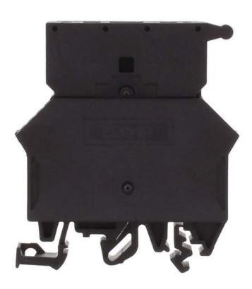
Fused terminal with disconnect plug, Screw connection, Mounting type:Mounting rail TS 35/7.5 and TS 32, Rated cross-section: 10 mm², Width: 10 mm, Colour: Black
