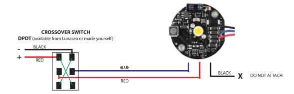
Using three wire setup apply power to either of the + leads - HI/LO or White/Red(Blue) capability
