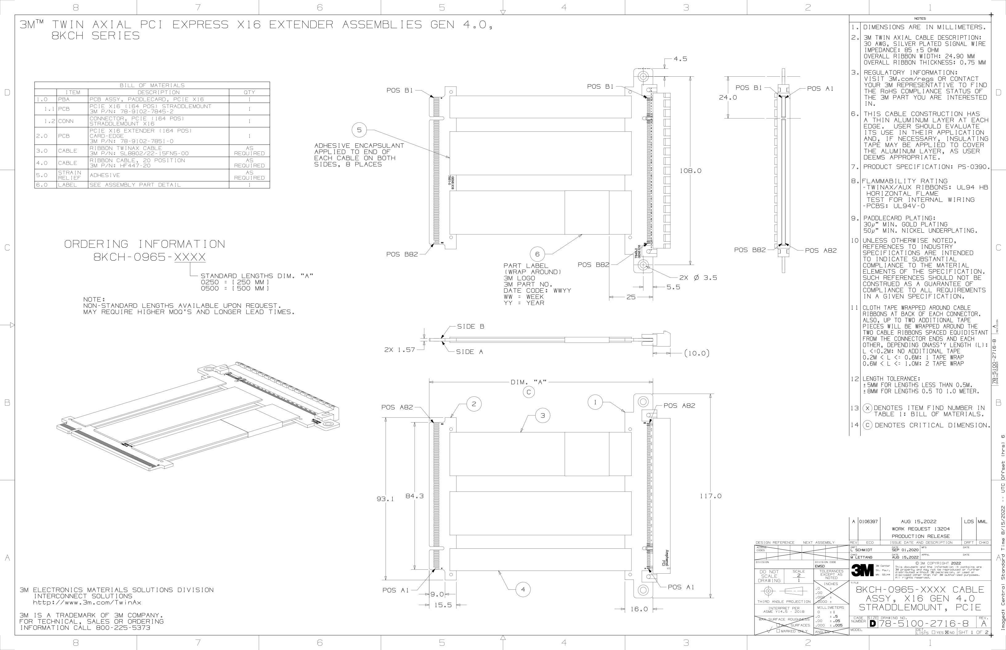
3M™ TWIN AXIAL PCI EXPRESS X16 EXTENDER ASSEMBLIES GEN 4.0, 8KCH SERIES CEM pin # Side A Description Name pin# A01 Presence detect PRSNT#1 A01 A02 A02 +12 volt power +12v A03 A03 +12 volt power +12v GND A04 Ground A04 A05 TCK JTAG2 A05 A06 TDI JTAG3 A06 A07 TDO JTAG4 A07 A08 TMS JTAG5 A08 A09 +3.3 volt power +3.3v A09 A10 +3.3 volt power +3.3v A10 PERST# A11 Fundamental reset A11 Mechanical Key A12 Ground A12 A13 Reference Clock, Differential REFCLK+ A13
