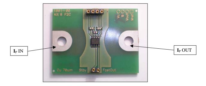
Connect then the primary between pins  $I_{\text{P}}$  IN and  $I_{\text{P}}$  OUT.
