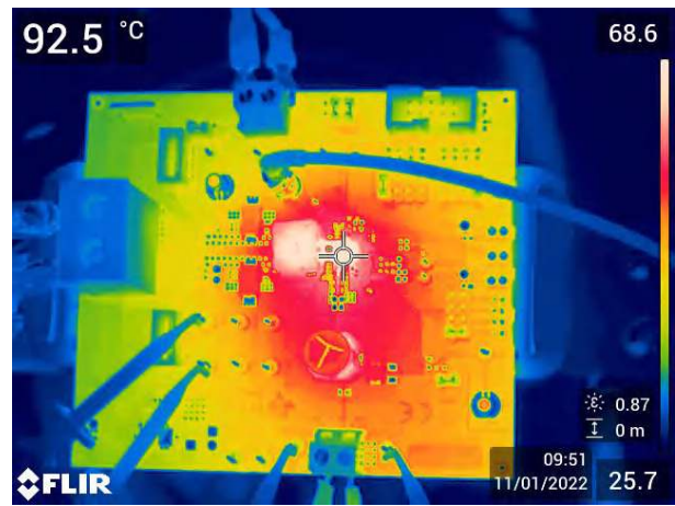
Figure 2-20. Thermal Characteristics, 600-kHz FCCM, External 5-V Bias, 35-A Load
