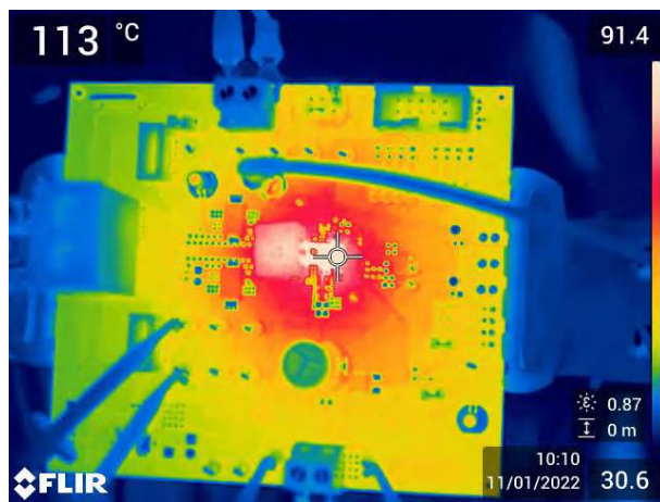
Figure 2-21. Thermal Characteristics, 800-kHz FCCM, Internal LDO, 35-A Load
