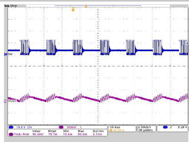
Figure 2-18. Output Voltage Ripple, DCM, 1-A Load
