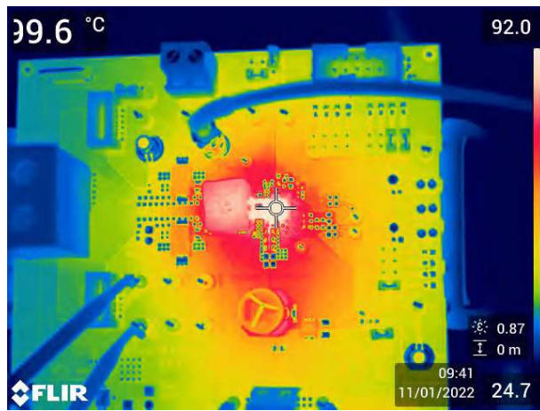
Figure 2-19. Thermal Characteristics, 600-kHz FCCM, Internal LDO, 35-A Load
