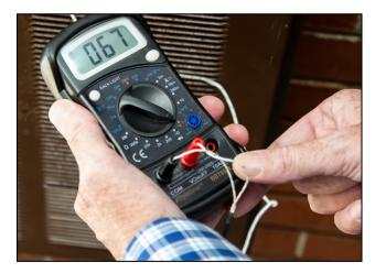
Includes K-type temperature thermocouple
