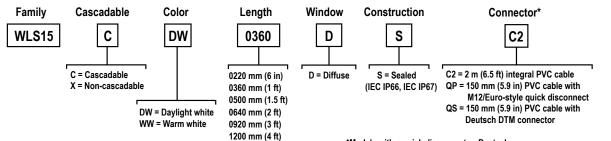
\*Models with a quick disconnect or Deutsch DTM connector require a mating cordset
