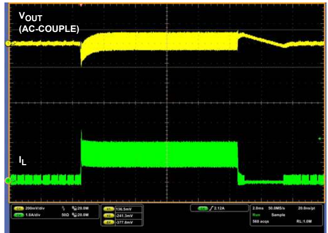
FIGURE 11. LOAD TRANSIENT RESPONSE 0A->1A, VIN = 36V
