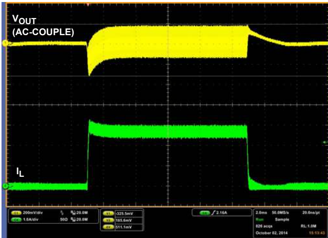
FIGURE 10. LOAD TRANSIENT RESPONSE 0A->1A, VIN = 8V
