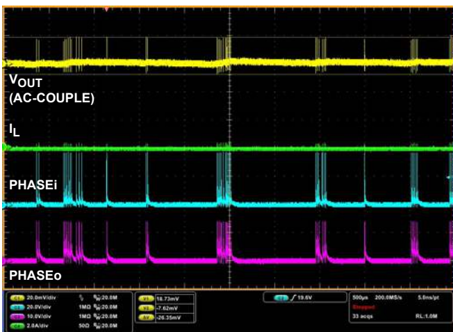
FIGURE 8. OUTPUT RIPPLE AT 0A LOAD ( V_{IN} = 36V )
