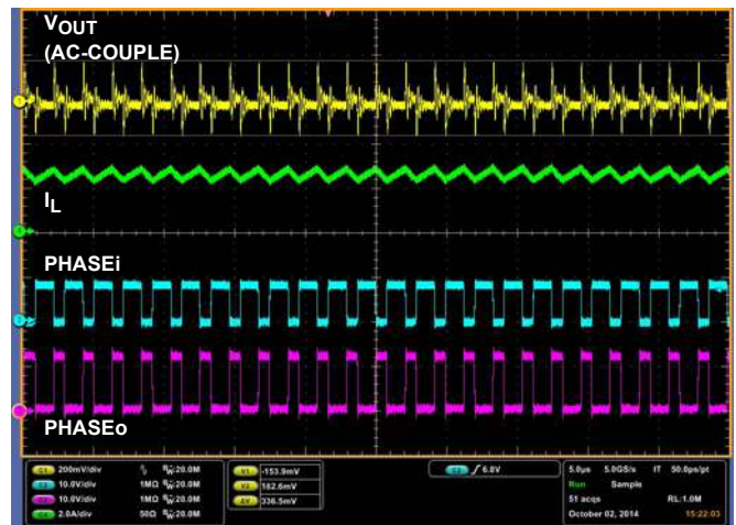
FIGURE 7. OUTPUT RIPPLE AT 1A LOAD ( V_{IN} = 8V )
