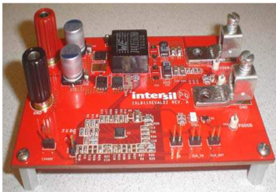
FIGURE 1. ISL8115EVAL2Z EVALUATION BOARD
