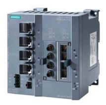
SCALANCE X308-2M PoE; managed IE switch, compact; 4x 10/100/1000 Mbit/s for RJ45 ports electrical with PoE; 2x 100/1000 Mbit/s for 2-port media modules, electrical or optical; LED diagnostics, error signaling Contact with select/set pushbutton, PROFINET IO device, network management, Integrated redundancy manager, office features (RSTP, VLAN, IGMP,...) C-plug in scope of supply.
