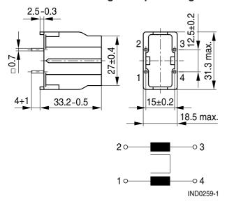
Part tolerances to ISO 2768-cL / ISO 8015. Size ISO 14405 (E) All dimensions in mm 1
