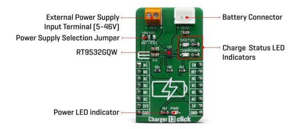
The RT9532GQW IC is designed with reliability in mind: the IC prevents draining the battery below the critical level, offers prequel charging (for deeply depleted batteries), features an overvoltage protection, charging status monitoring and so on. The Click board™ itself is equipped with a set of indicators used to monitor both charging process and power distribution.
