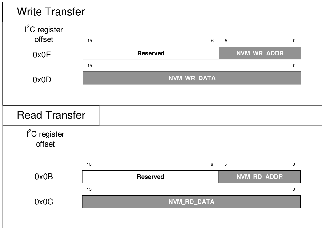
Figure 9-12. EEPROM Direct Access Using I 2 C
