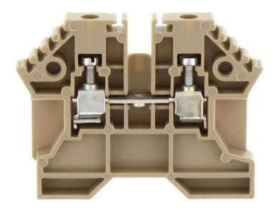
Feed-through terminal for direct mount/block variant, Screw connection, Mounting type: Mounting surface, Rated cross-section: 2.5 mm<sup>2</sup>, Width: 5 mm, Colour: Beige
