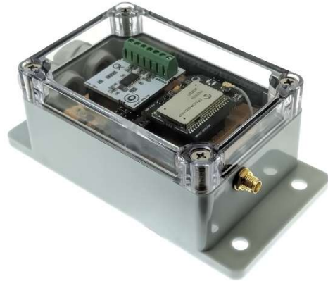
Pic. 23. Beehive LoRa monitoring system
