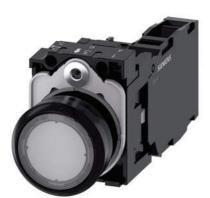
Illuminated pushbutton, 22 mm, round, plastic, clear, pushbutton, flat, momentary contact type, with holder, 1 NO+1 NC, LED module with integrated LED 110 V AC, screw terminal
