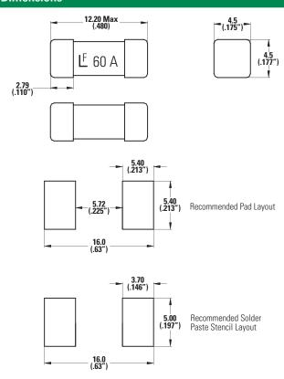
Note: Recommended Stencil Thickness: 0.152 mm Dimensions are in millimeters (inches)
