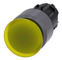
Illuminated mushroom pushbutton, 22 mm, round, plastic with metal front ring, yellow, 30 mm, latching, pull-to-unlatch mechanism, with laser labeling, lower case
