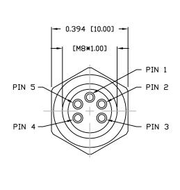
NOTE: MATERIAL HDUSING: PBT UL94V-0, BLACK CONTACT: BRASS SHELL **BRASS** NUT: BRASS □-RING: EPDM, BLACK FINISH: GOLD PLATED CONTACT: **OVER 50u" NICKEL** SHELL: NICKEL NUT: **NICKEL** ELECTRICAL 1.5A RATED CURRENT: 30∨ RATED VOLTAGE: INSULATION RESISTANCE: 100 MOhms MIN. CONTACT RESISTANCE: 10 mOhms MAX. WATER PROOF: IP67 **ENVIRONMENT OPERATION TEMPERATURE:** -40°C TD +85°C MAX WIRE AWG: 26
