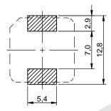
no sensitive traces underneath the component
