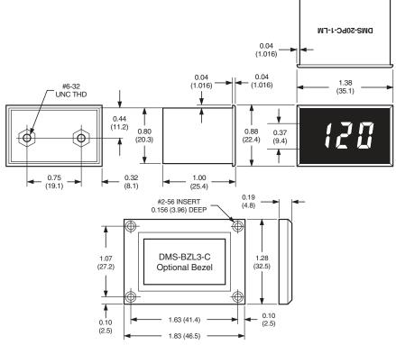
Dimensions in inches (millimeters) Tolerances: 2 PL Dec ±0.02 (±0.51) 3 PL Dec ±0.010 (±0.254) Recommended panel cutout dimensions: 1.336 (33.93)W × 0.838 (21.29)H Internal corner radii 0.032 (0.81) Max.
