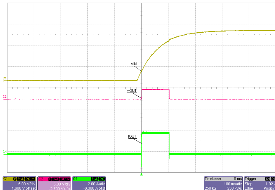
Figure 6. J9 = NO Jumper Current Limit Test with Latch (CH2)
