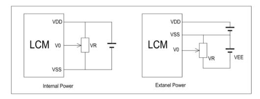
VDD-V0: LCD Driving Voltage VR: 10k-20k
