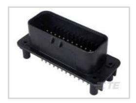
Connector System: Wire-to-Board Number of Positions: 35 Centerline (Pitch): 4 mm [.157 in ] Sealable: Yes PCB Mount Orientation: Vertical All AMPSEAL PCB Headers (58)
