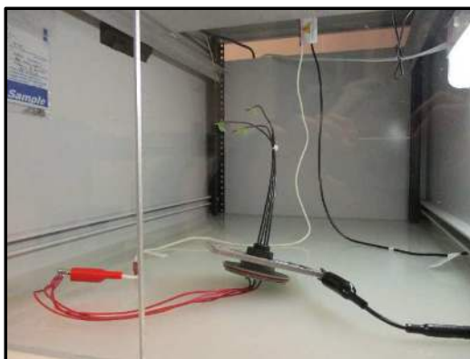
Figure 16 – Typical Withstanding Voltage – External Setup
