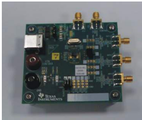
Figure 2. CDCS502 Printed-Circuit Board
