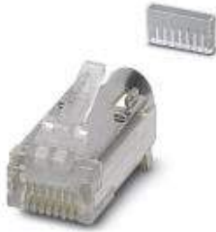
RJ45 pin insert, CAT5e, 8-pos., shielded, IDC connection method, for litz wires AWG 27 ... 26, with strain relief
