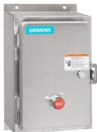
Non-reversing motor starter Size 1 Three phase full voltage Solid-state overload relay OLRelay amp range 10-40a 110-120/220-240VAC 60HZ coil Combination type Water/dust tight non-corrosive
