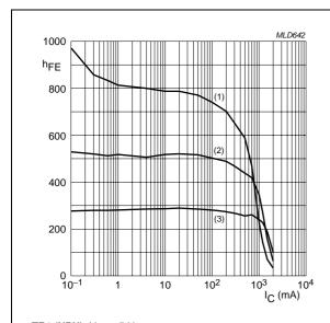
**TR1 (NPN);**  $V_{CE} = 5 \text{ V}.$
