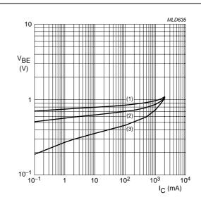
**TR1 (NPN);**  $V_{CE} = 5 \text{ V}.$
