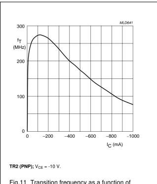
Fig.11 Transition frequency as a function of collector current; typical values.
