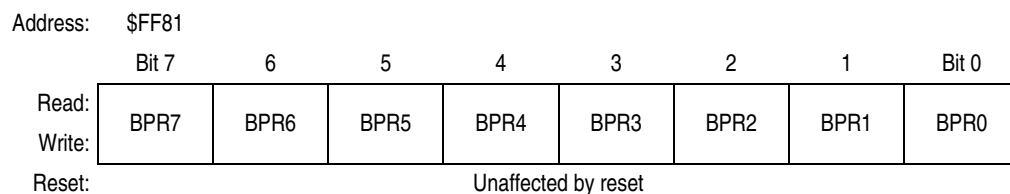
Figure 2-8. FLASH-2 Block Protect Register (FL2BPR)
