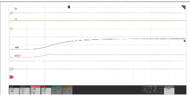
R_{OVCSSEL} = \text{Open} , C_{OUT} = 220 \mu F , I_{OUT} = 200 \text{ mA} , V_{IN} ramped up from 5 V to 7.5 V
