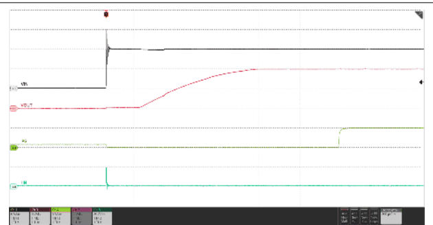
C_{OUT} = 22\ \mu\text{F} , C_{dVdt} = \text{Open} , EN/UVLO connected to IN through resistor ladder, 12 V hot-plugged to IN
