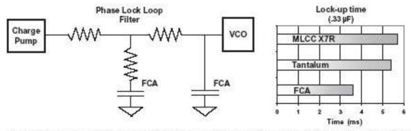
FCA surface mount film capacitors have advantages over tantalum and ceramic capacitors in PLL circuits. There are no piezoelectric effects to create noise, they are not polarized, and they result in faster signal lock-up time.
