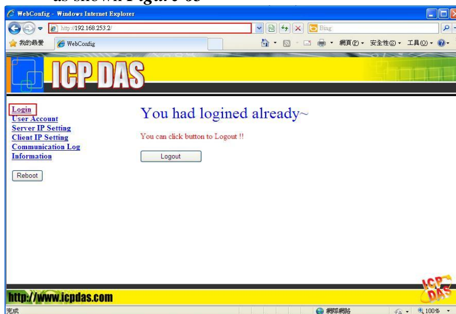
Figure 63 Browser the Web of I-7550E and enter the default password to login.
