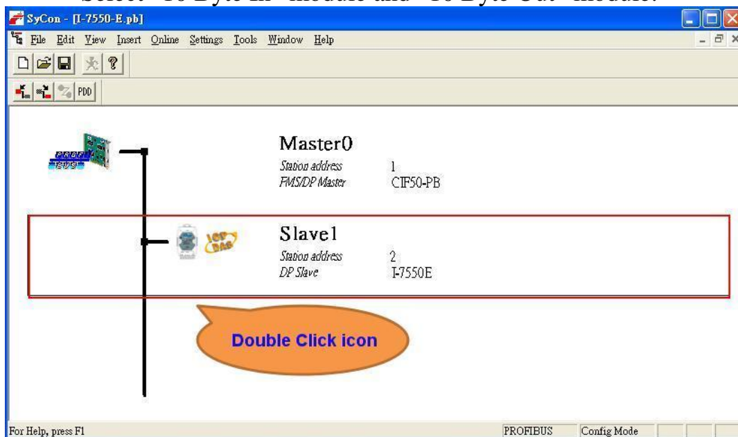
Figure 45 Double click the I-7550E icon to open the “Slave configuration” window
