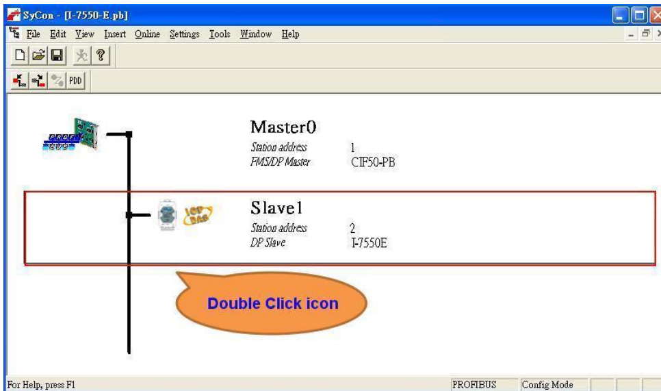
Figure 73 Double click the I-7550E icon to open the “Slave configuration” window
