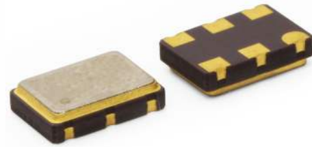
Part Dimensions: 7.0 × 5.0 × 2.0mm • 178.462mg
