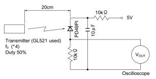
In the above figure, the transmitter should be set so that the output V<sub>OUT</sub> (P-P) can be 40mV. However, the PD49PI to be used here should be of the short-circuit current Isc=2.6  $\mu$  A at Ev =100 Ix. (Ev is an illuminance by CIE standard light source A (tungsten lamp).)
