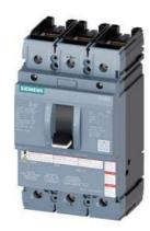
molded case switch 3VA5 UL frame 250 max. sh-circ breaking capacity 100kA @ 480 V 3-pole, line protection MCS110, In=100A without overload protection self-protection Ii=25 x In cable connection on both sides
