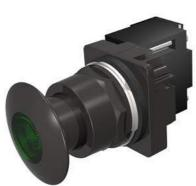
30mm BlackMax, Epoxy Coated Corrosion Resistant Complete Metal Unit Illuminated Push-Pull Operator Full Voltage, 24V AC/DC Incandescent Lamp Mushroom Head Cap Small 1 3/4" (44.5 mm) Metal, Black with Green Lens 3 Position Momentary UL Listed, CSA Certified NEMA 1,3,3R,4,4X,12,13 & Automotive Standards
