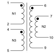
N2 denotes two windings connected in parallel. Terminals 6+7 and 9+10 must be tied as solder bridging is allowed.
