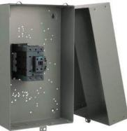
Electrically held lighting contactor, Contactor amp rating 100A, 0 N.C. / 3 N.O. Poles, 480VAC 60HZ coil, 1 NO / 1 NC auxiliary contacts Non-combination type, (no disconnect device), Enclosure NEMA type 1, Indoor general purpose use
