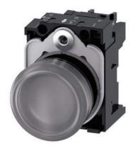
Indicator lights, 22 mm, round, plastic, clear, lens, smooth, with holder, LED module, with integrated LED 230 V AC, screw terminal  $\,$
