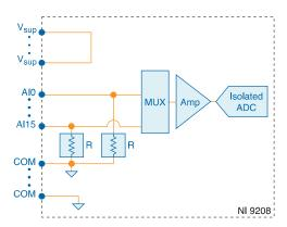
The input signals are scanned, amplified, conditioned, and then sampled by a single 24-bit ADC. The module provides overvoltage protection for each channel. Only one channel can be in an overvoltage condition at a time.
