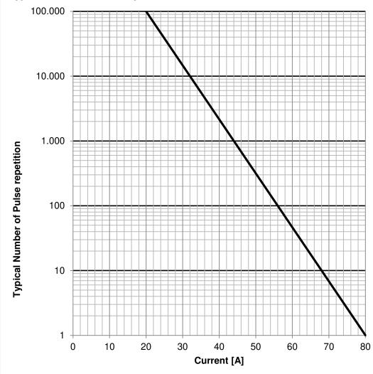
valid for ambient temperature: +25°C; 8 ms pulse length, 10 s break between pulse
