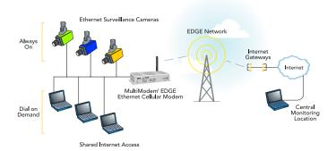
Industry-standard Modem Commands. The MultiModem EDGE cellular modem provides industry-standard AT-style commands for ease of integration into your existing software application.
