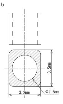
\* Nozzle with chamfering is recommended
