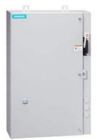
Non-reversing motor starter Size 4 Three phase full voltage Solid-state overload relay OLRelay amp range 50-200A 190-220/220-240V 50/60HZ coil Combination type 150A circuit breaker Enclosure NEMA type 4/12 Water/dust tight for outdoors Standard width enclosure
