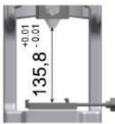
Verify that the press and the mini applicator's axis are perfectly in line.
