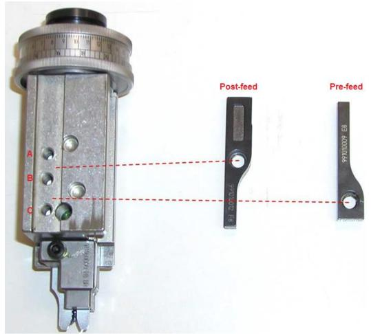
Moving the post-feed cam from B to A changes the stroke from 40 to 30 mm. Moving the pre-feed cam from C to B changes the stroke from 40 to 30 mm.
