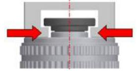
Set the top ring of the continuous adjusting head in accordance with the data on the identification plate.
