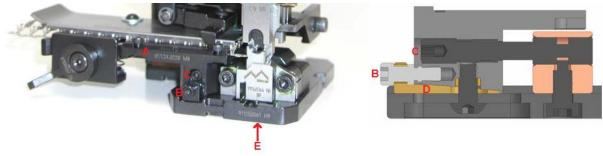
For adjusting the bellmouth, loosen the screw B to release the wedge D and the terminal slide A. Rotate screw C clockwise or counter-clockwise to obtain the desired adjustment. Tighten B again until D blocks A.
