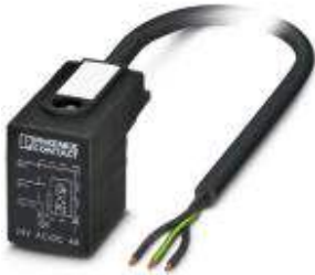
Sensor/Actuator cable, 3-position, PVC, Black RAL 9005, Free cable end, on B valve plug (10 mm), with 1 LED, connected with Z diode, Cable length: 5 m
