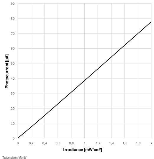
Testcondition: Ee=0,5mW/cm<sup>2</sup>, VR=5V
