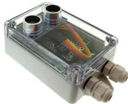
Pic. 15. WiFi Ultrasound sensor : waste collection project
