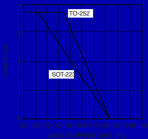
Figure 9. Maximum Power Dissipation
